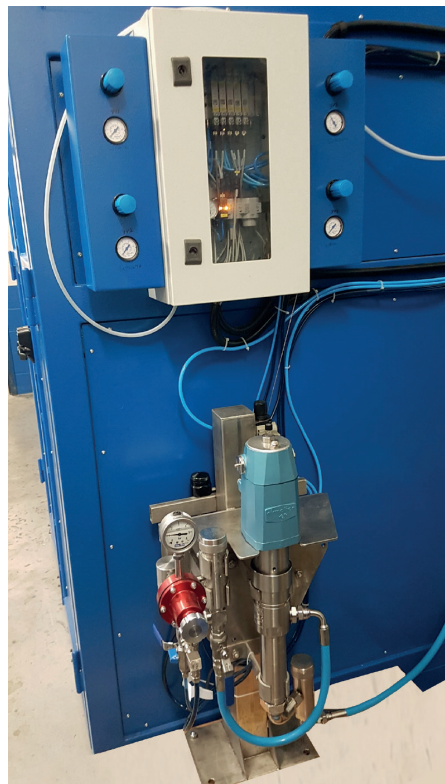
↑ Feeding system, multi-stage filtration and pressure control
