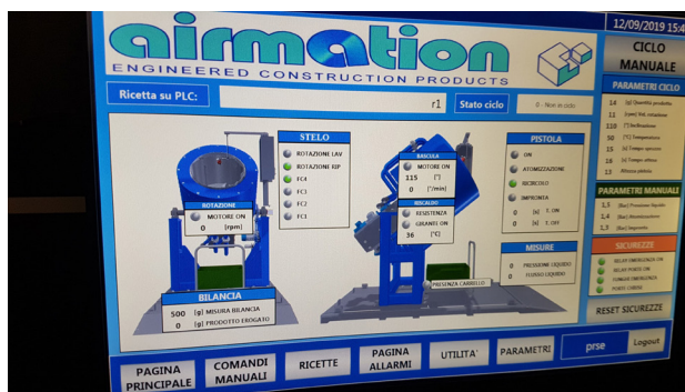
↑ The operator panel allows programming of recipes, displays alarm situations and allows the machine to be controlled
